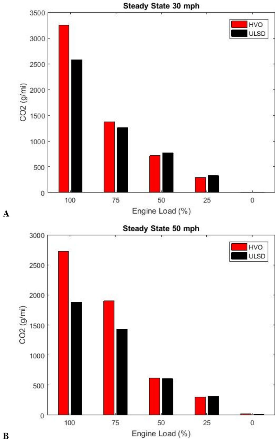
**Figure 3-12 (a-b):** CO<sub>2</sub> emissions over the steady-state 30 mph (A-top panel) and 50 mph (B-bottom panel) conditions
