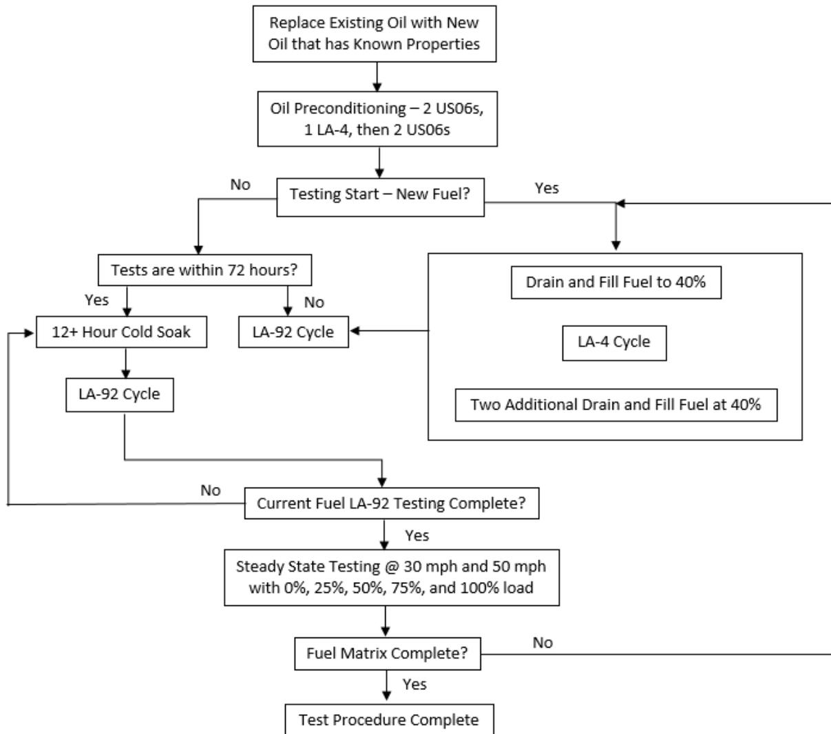
**Figure 2-3:** Test sequence for fuel change procedure and oil conditioning
