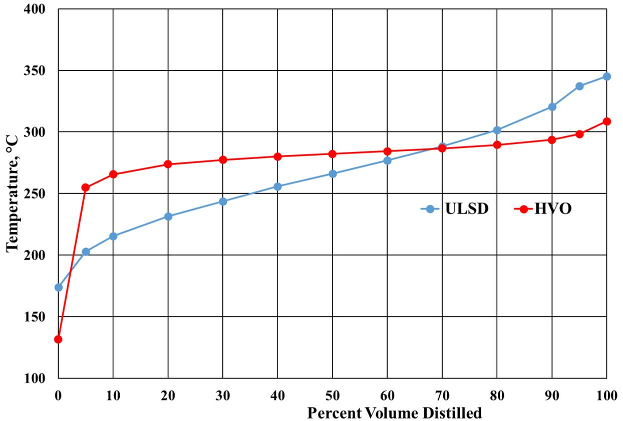
**Figure 2-1:** Distillation characteristics of the ULSD and HVO fuel using the ASTM D86 method
